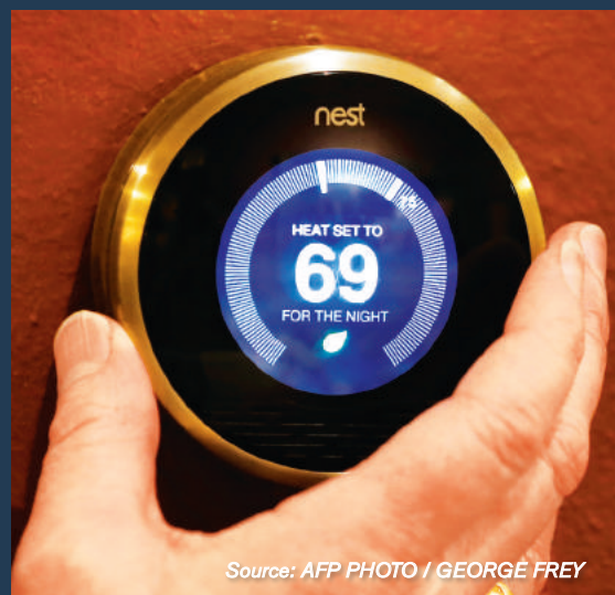
The Alphabet 'Nest', a smart thermostat that adjusts temperatures by analysing the daily habits of occupants at home to reduce energy consumption.
