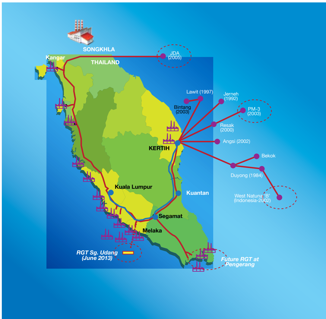
Figure 4: Natural Gas Sources and Peninsular Gas Utilisation (PGU) System
