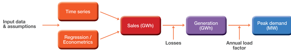
Figure 16: Process flow of electricity demand forecasting analysis
