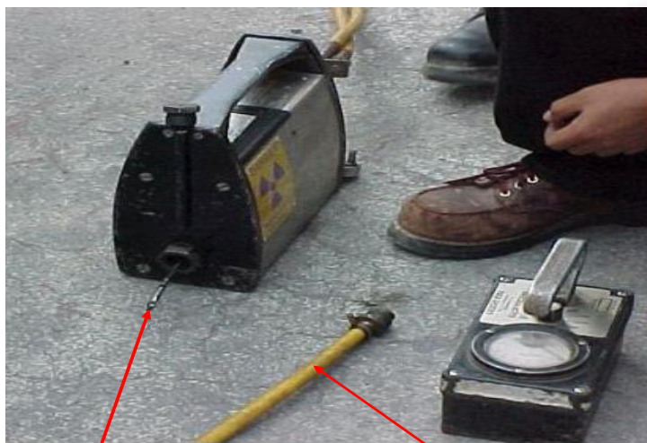
Broken male connector (connecting radioactive source capsule with winding cable)
