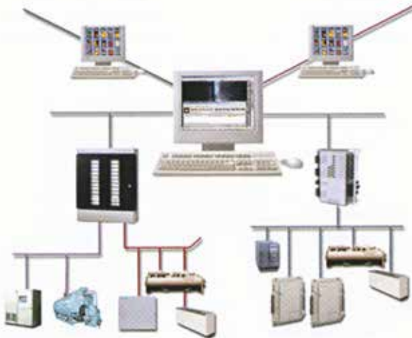
Building Energy Management System used to control, manage and monitor the energy consumption in buildings
