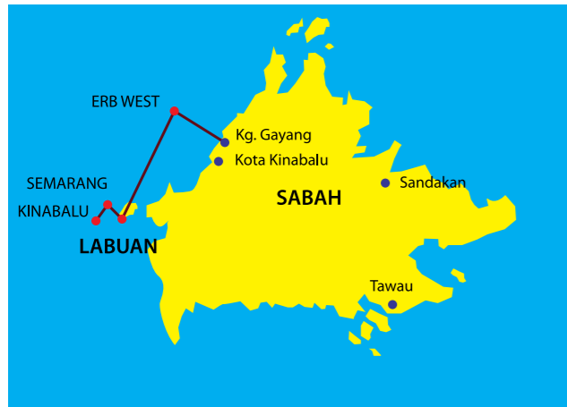
Rajah 2.5: Sistem Pengagihan Gas Asli di Sabah dan Labuan Figure 2.5: Natural Gas Distribution System in Sabah and Labuan
