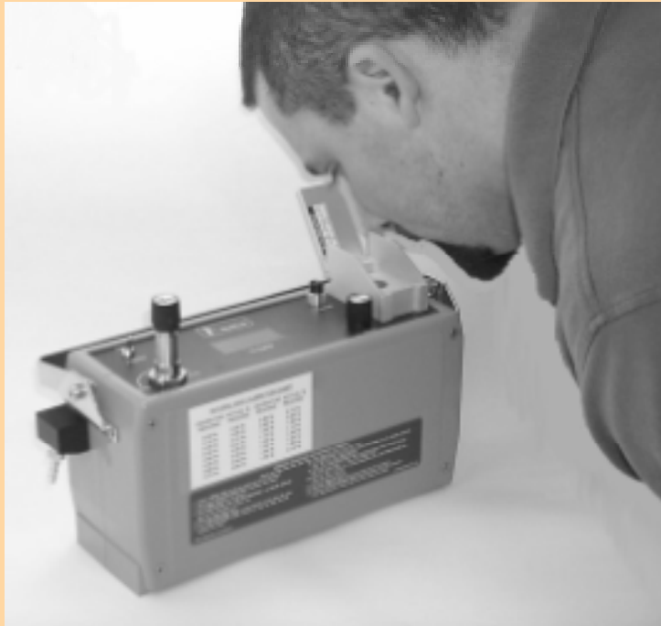
Figure 4.6: The “Smelling” Process of Odorator for Gas Detection
