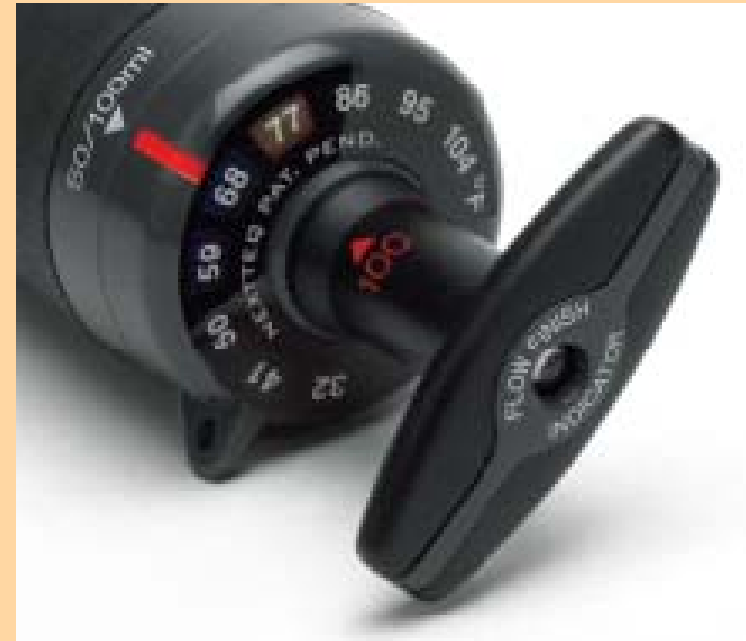
Figure 4.3: Length of Stain Tubes and GASTEC Precision Pump
