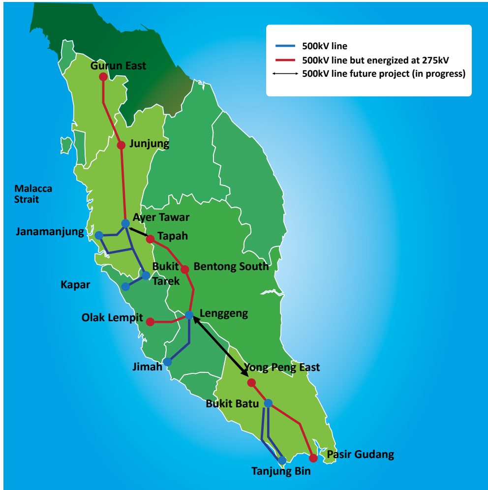
Figure 19: 500kV transmission line from Ayer Tawar to Tapah and Yong Peng East to Lenggeng
