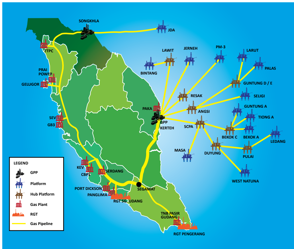
Figure 3: Gas supply infrastructure in Malaysia
